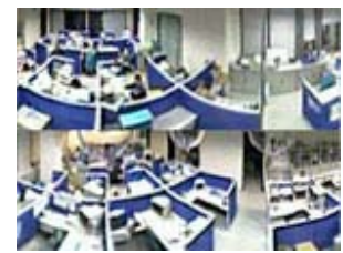
Two 180° split views of cylinder projection de-warping
